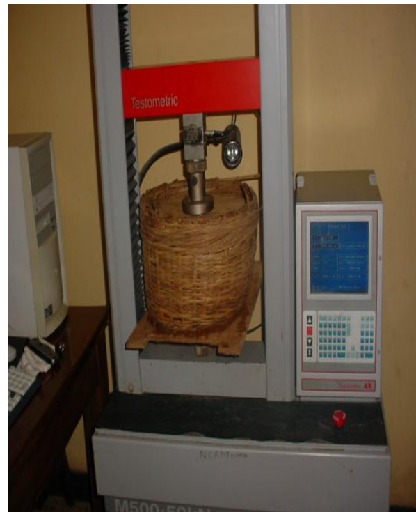
Fig. 1. Compression of Roma tomatoes in raffia basket using Testometric Universal Testing Machine. (UTM).
